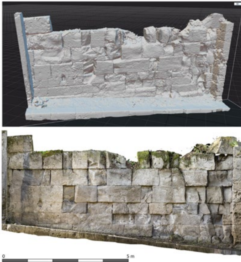
Fig. 6. Three-dimensional model of the surfaces (Digital Surface Model) and their relative orthophoto
