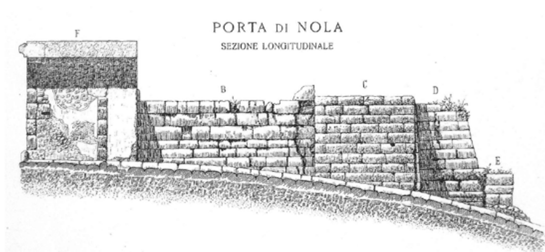
Fig. 15. Porta Nola, longitudinal section by Maiuri, 1930, Tav. XI
