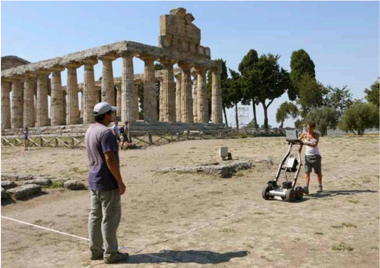
Fig. 4. View of the prospection survey done by Federica Boschi and Michele Silani; the method used is ground penetrating radar (GPR). (photo R.M. Ammerman)
