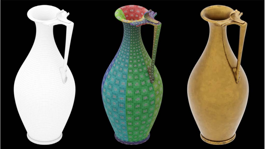
Figure 1. 3D modelling. (a) solid mesh; (b) uv unwrap; (c) textured mesh.
